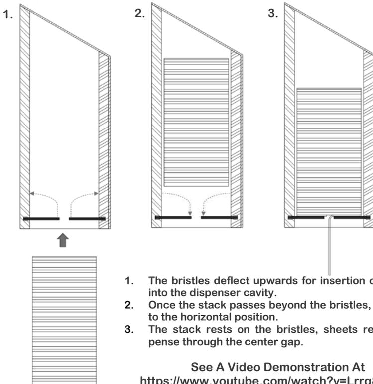
1. The bristles deflect upwards for insertion of the stack into the dispenser cavity.
